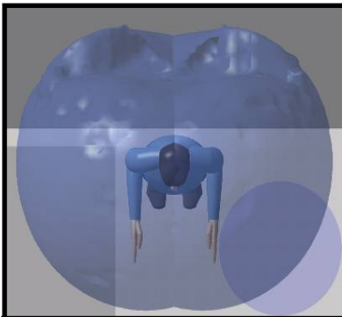
Figure 5: Displays the 3D geometry generated from the human model's reach envelope
